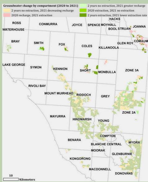
When applied to 2020 and 2021 data FORETHIR finds that, even within model error, the rates of extraction for both softwood and hardwood plantations are generally lower than the deemed rates of the Lower Limestone Coast Water Allocation Plan and significant areas of recharge are predicted to occur across the region, consistent with the findings of other methods.
