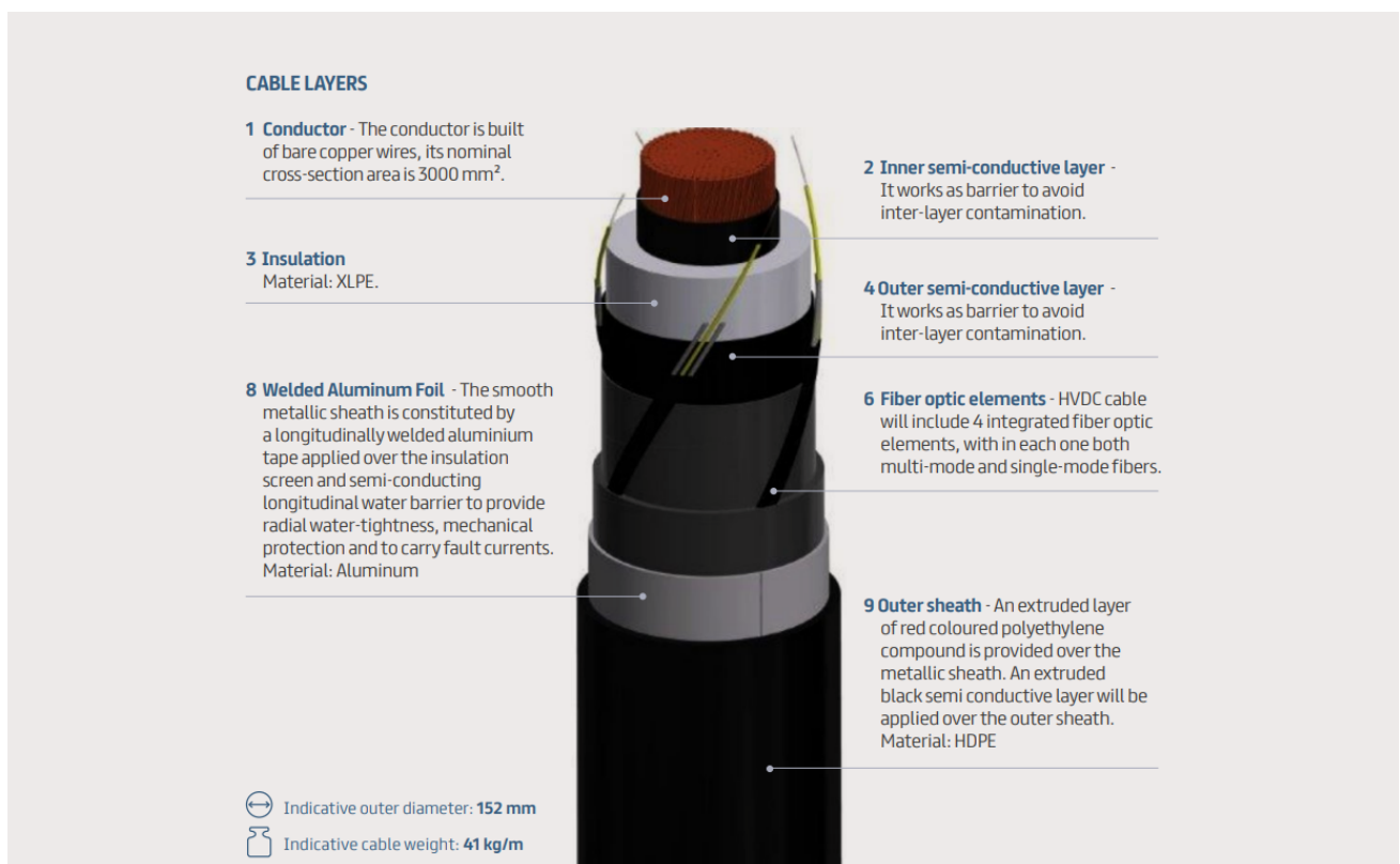
Figure 29. Suedlink HVDC XLPE Cable (Prysiam Group [26]).
