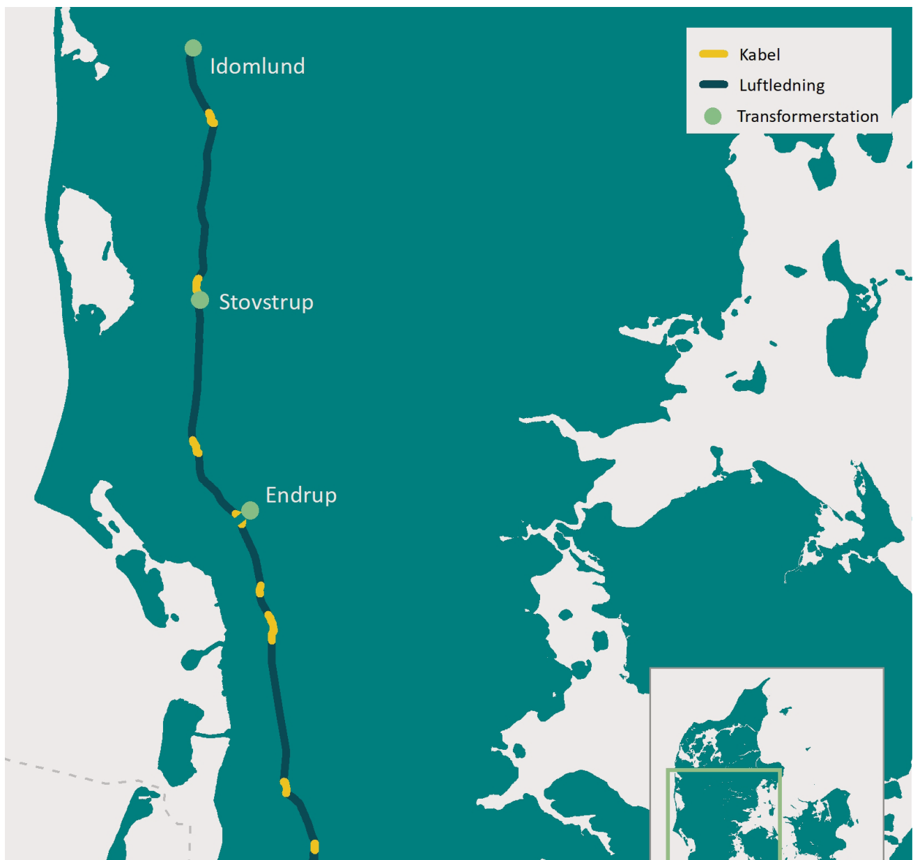
Figure 11. Overview Map of West Coast 400kV AC Interconnector Idomlund Denmark to Germany (Energinet)
