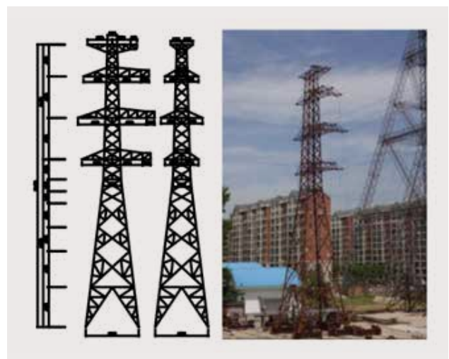
Figure 4 – General map of double circuits 110STJ tower [11]
