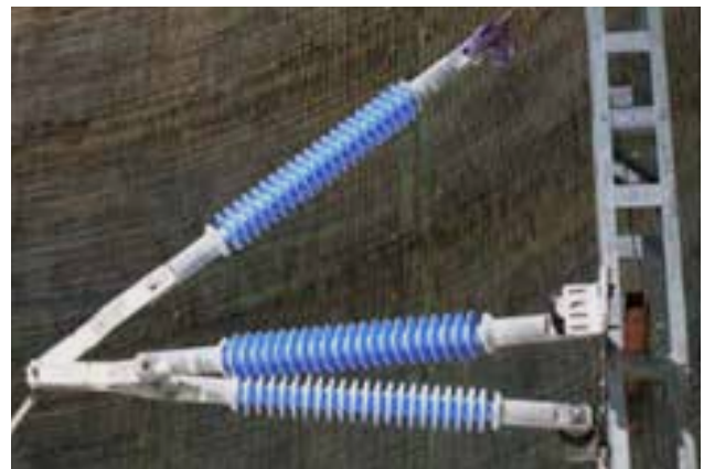
Figure 6 – Photo of the insulator set-up for pollution tests [23]
