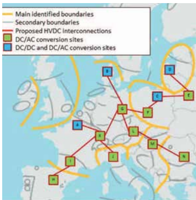
Figure 10 – A possible hybrid AC/DC transmission network proposal [14]
